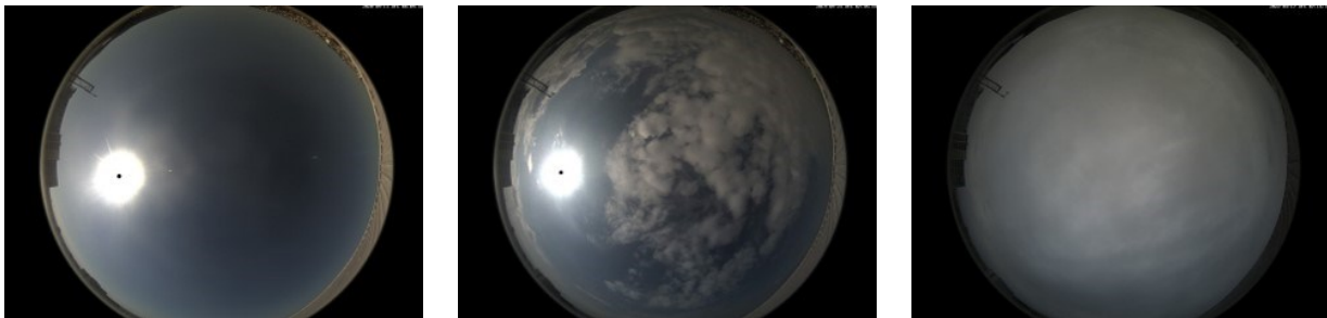
Figure 2. Sample images captured the sky-camera at LAP/AUTH under different cloud conditions (left: clear-sky; middle: broken clouds; right: overcast). Numerous collocated ground-based and satellite data are available since the sky-camera stores an image of the whole sky every 1 minute (hence also during S5P overpasses) and therefore the time difference between the two instruments would be negligible. High NO 2 concentration levels are not infrequent at LAP/AUTH, especially during the cold period. The synergy of the sky-camera and the MAX-DOAS systems will make available the identification of the required highly NO 2 polluted cases under different cloud conditions, that are mentioned above, for the evaluation of the improved algorithm for 3D cloud handling.
