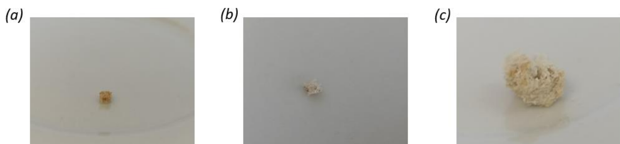
Figure 3. a) Ceramic foam derived from Silk Fina template, b) Ceramic foam derived from Hard template and c) Ceramic foam derived from Honeycomb template.
