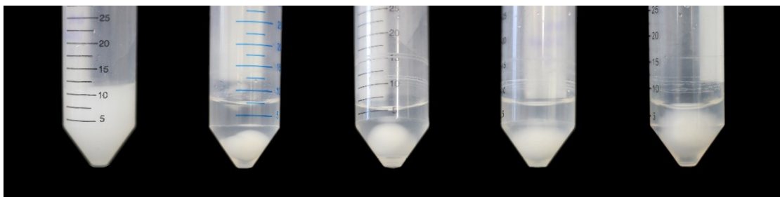
Figure 2. Czapek-Dox medium with 0.4% (v/v) Impranil® DLN-SD inoculated with the strains #964, 0834, 965, 970, 960 (from left to right) after 18 days of incubation in liquid cultures at 25°C, under agitation (80 rpm). Strain #964 (left) shows neither growth nor polymer degradation ability compared to the other strains.
