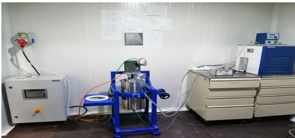
Figure 1. Carbon dioxide hydrate formation reactor connected with control unit (left) and cooling bath (right)
